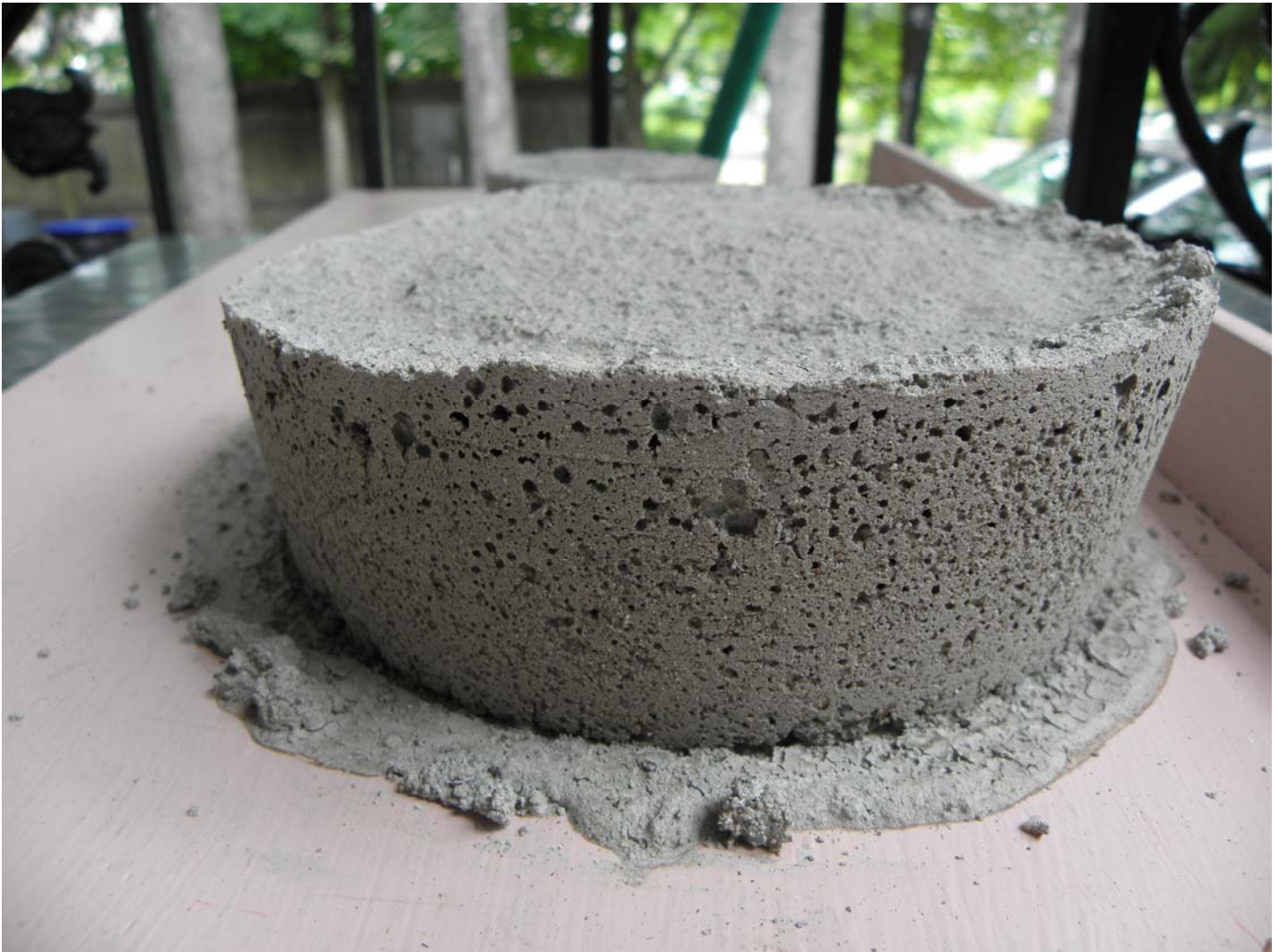
Day Four (large sample) Air pockets are visible because of hand compacting
