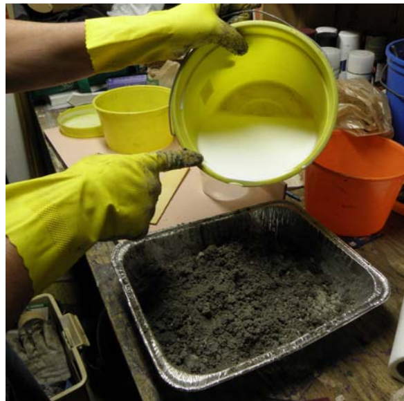
Mixture of Aggrebind and water being added to ground concrete
