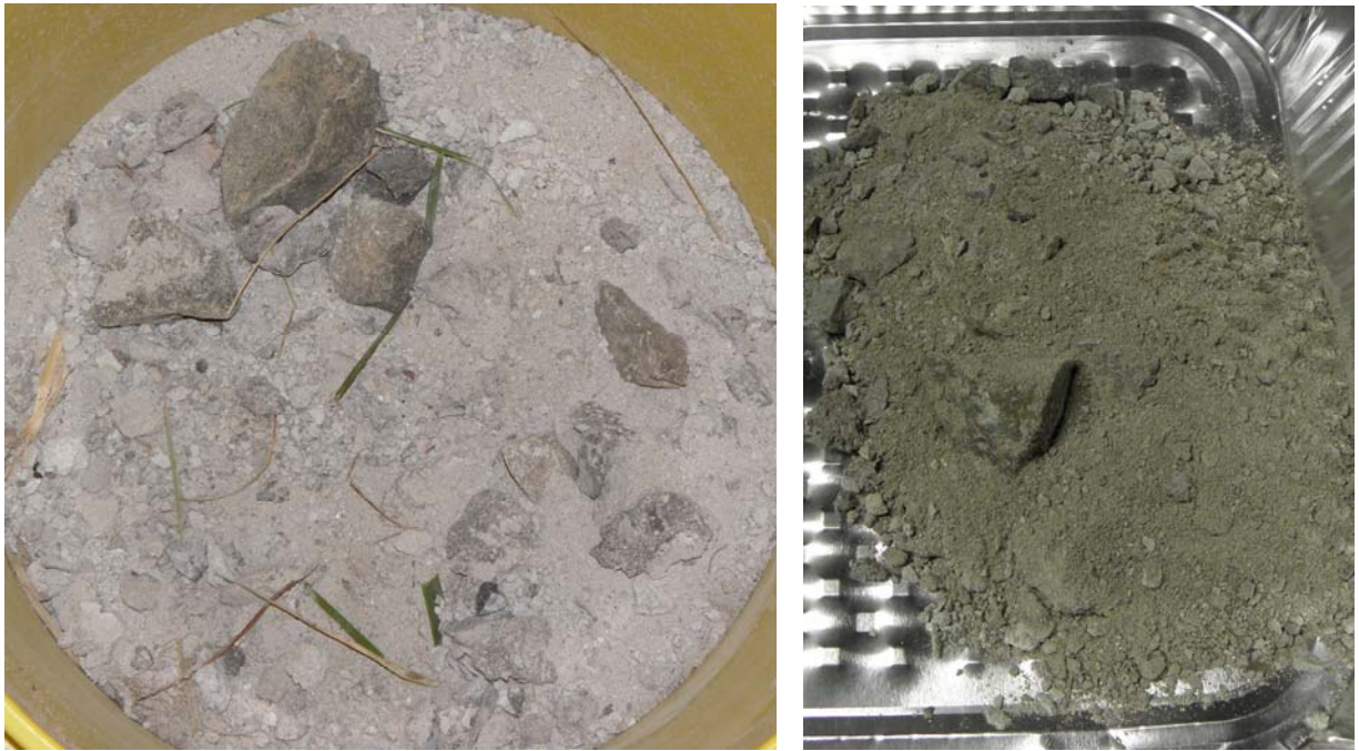
Ground or pulverized concrete (left), Removed all organic material (right) and larger rocks, fines not to exceed 30% of total depth
