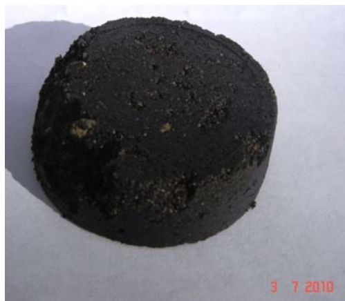
Pic 5 Tar-sand residue blended with AGGREBIND
